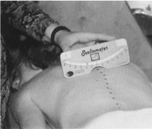
Figure 4.11 The OSI scoliometer used to measure the ATI in the spine of a scoliosis subject lying prone.
