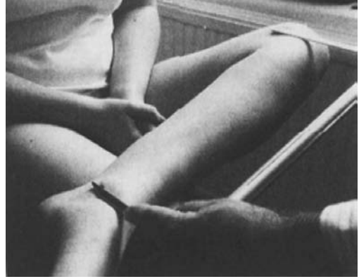
Figure 4.4 Holtain anthropometer used to measure tibial length. A counter recorder is employed, which gives an instant and accurate read-out of length.
