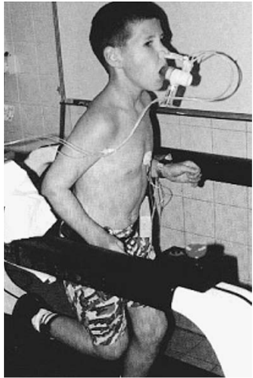
Figure 6.2 One of the children from the study by Eston et al. (1998). He is wearing the Tritrac on his left hip, the ActiGraph accelerometer on his right hip, a heart rate monitor (BHL 6000 Medical) and three pedometers: one on his right hip, one on his left wrist and one on his right ankle.
