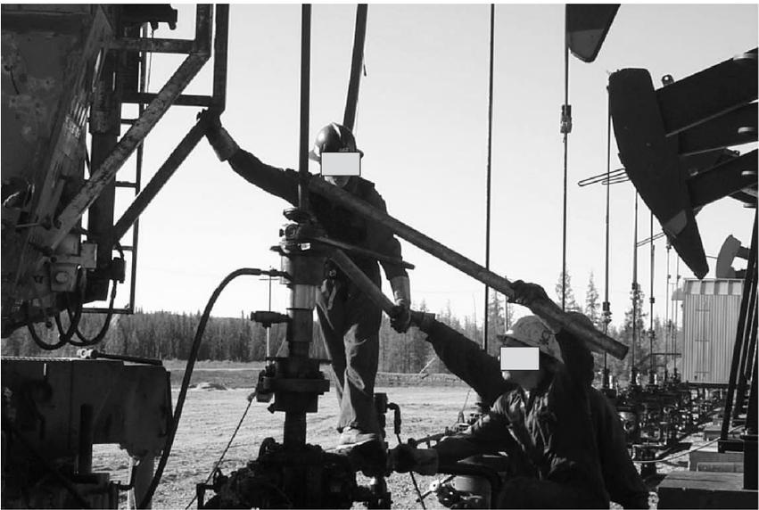
**Figure 6-19** Operator using an 8-ft extension to increase the force applied to a well-head block.
