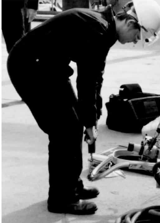
**Figure 3-1** Using a force gauge to measure a pushing/pulling task.
