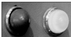
Off (left) and On (right) status lights on a control panel
