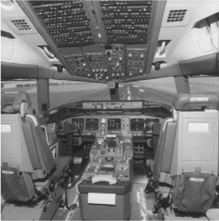
Figure 13.1 A modern aircraft flight deck simulator (reproduced by permission of Thales Simulation)
