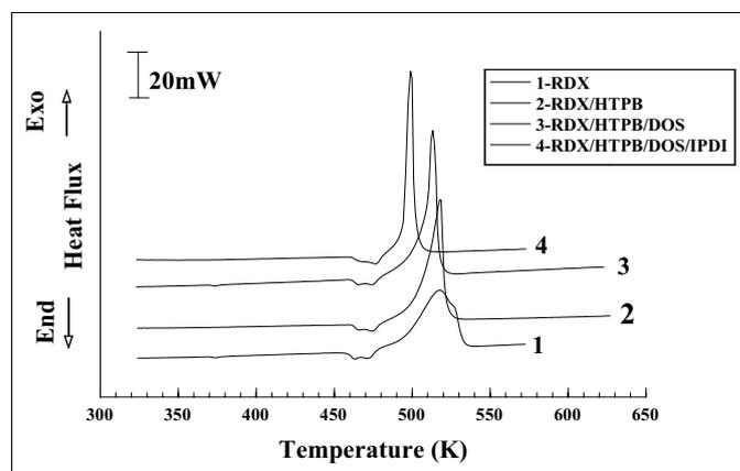
**Figure 3.** Typical DSC curves for PBX based on RDX at a heating rate of 10 K.min<sup>-1</sup>.
