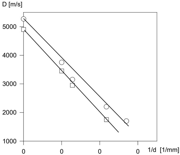
Fig. 2c. Diameter - effect curves for AN/TNT 90/10
