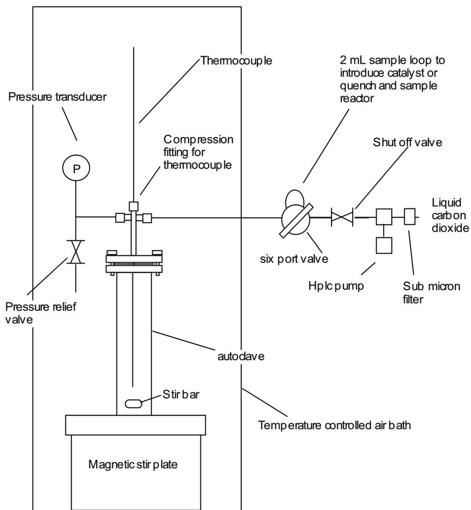
**Figure 2. Improved Experimental Apparatus with Temperature Control of all High Pressure Parts and a 6 Port Sampling Valve**
