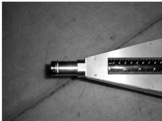
Figure 2. Ionization chamber with  $2\ \mu\text{g}$   $^{252}\text{Cf}$  source and preamplifier coupled to a pyramidal shielding, consisting from layers of iron, polythene and lead.
