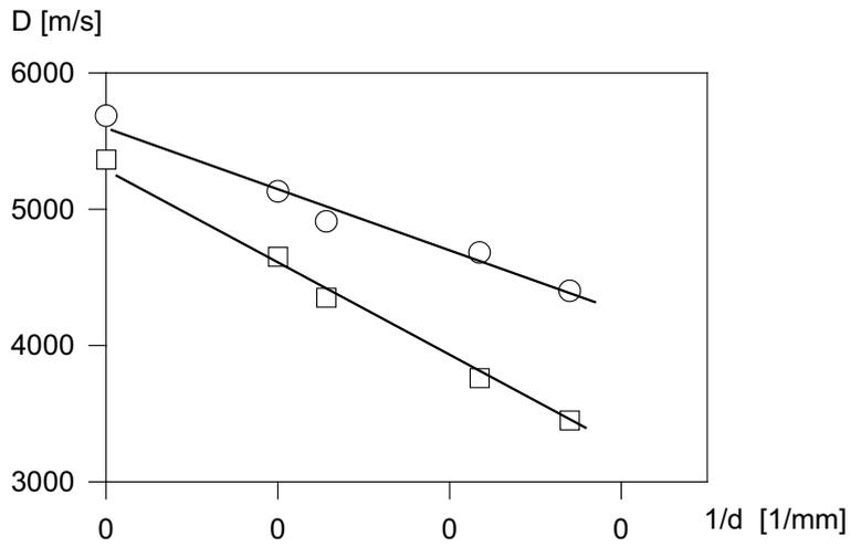
Fig. 2b. Diameter - effect curves for AN/TNT 60/40
