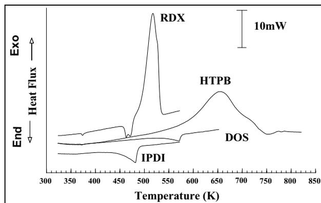
**Figure 1.** Typical DSC curves of individual compounds for an heating rate of  $10 \text{ K}\cdot\text{min}^{-1}$ .
