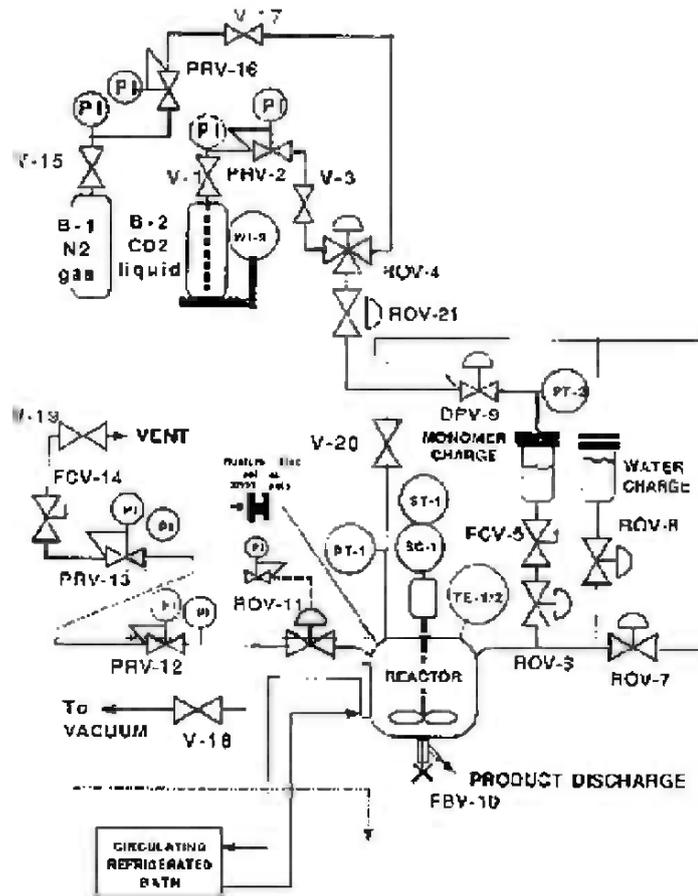
**Figure 2. Modified Reactor Design and Support Equipment**
