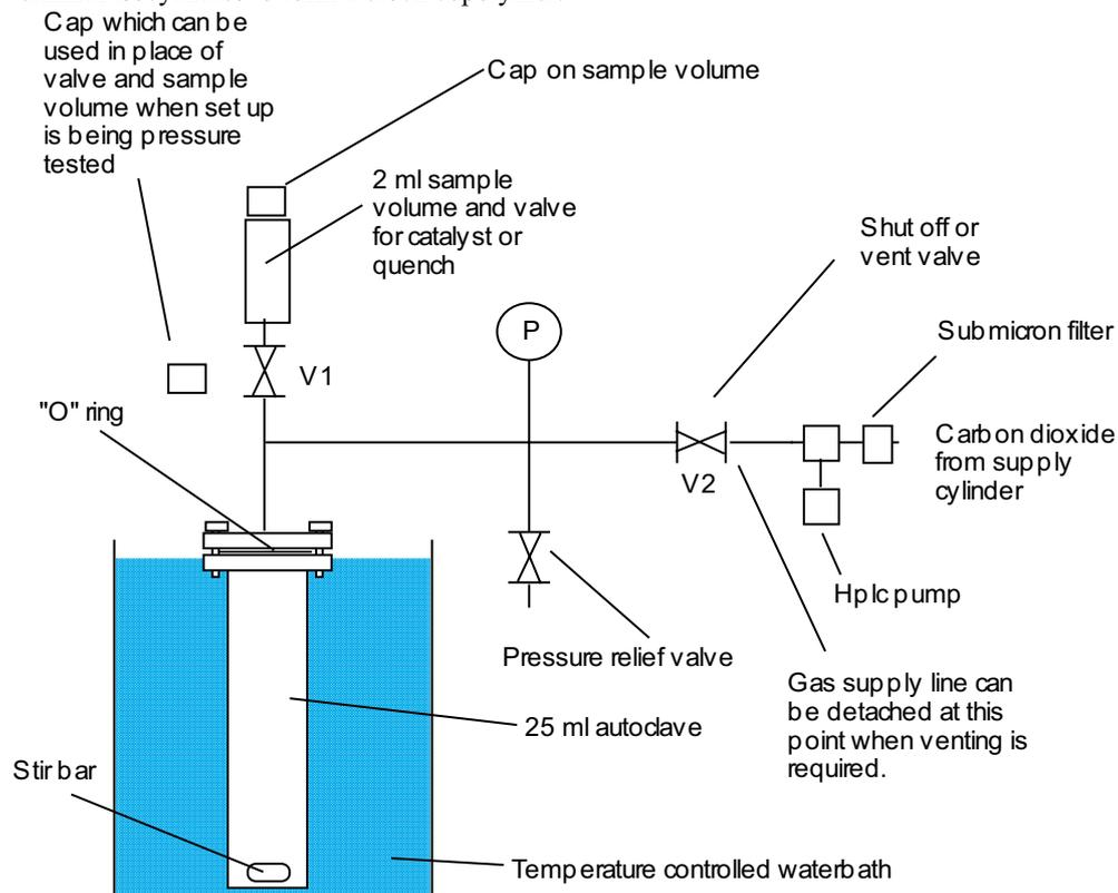
Valves V1 and V2 are rated to retain a system pressure of 2500 psi when exposed to atmospheric pressure on the discharge side
