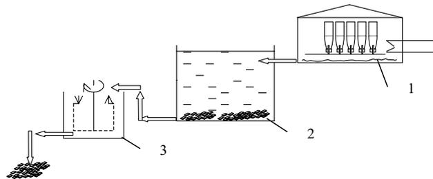
Fig.1. Sketch of the process line for melting down and granulation of TNT:
