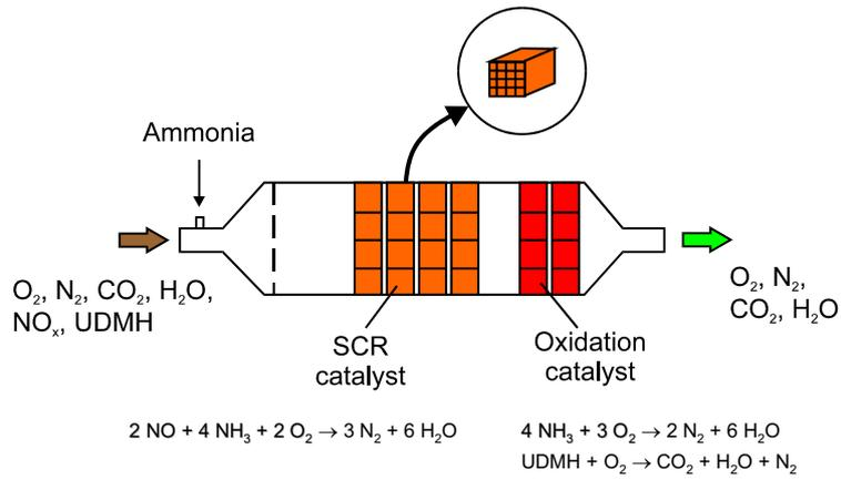
Flow diagram of the pilot plant for UDMH catalytic fluidized bed destruction
