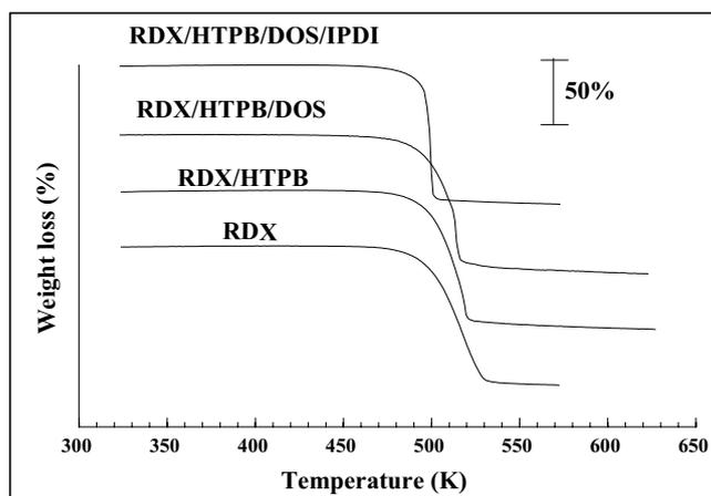
**Figure 2.** Typical TG curves for PBX based on RDX at an heating rate of  $10 \text{ K}\cdot\text{min}^{-1}$ .
