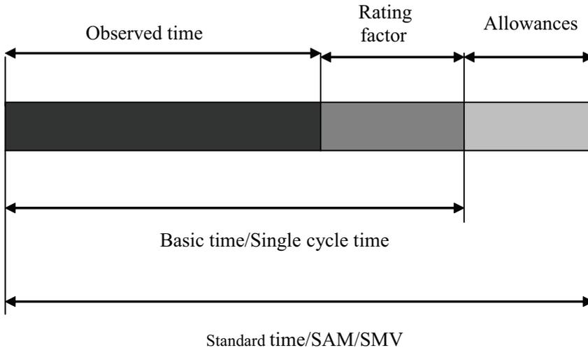
6.6. How the standard time for a simple manual job is made up
