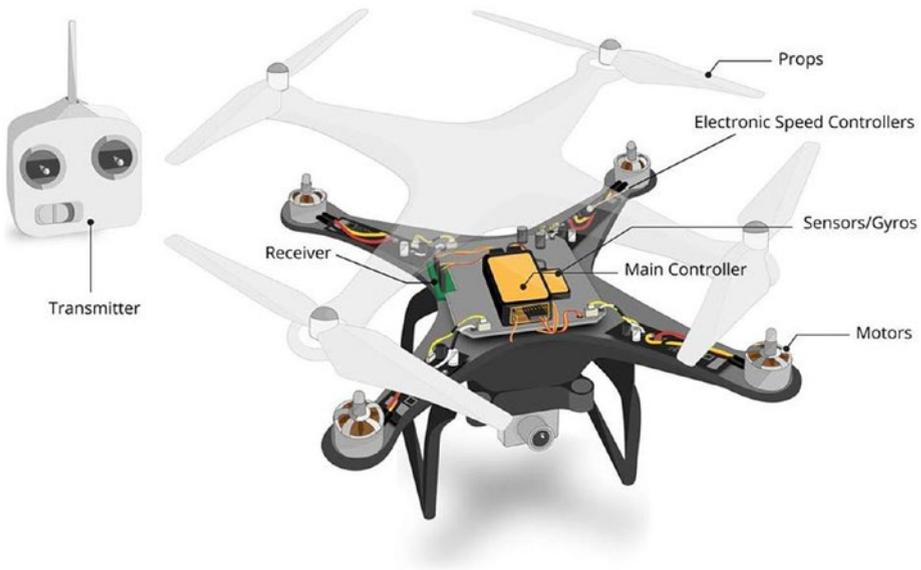
**Figure 1-4.** *Parts of a drone*
