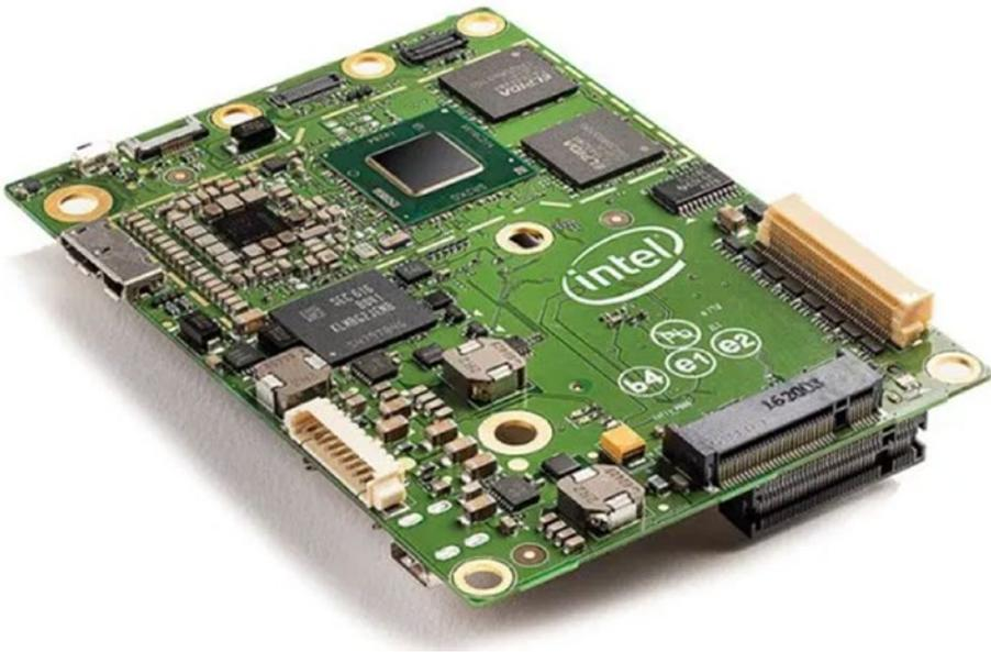
**Figure 1-2.** PCBA mounted with SOC and subsystems
