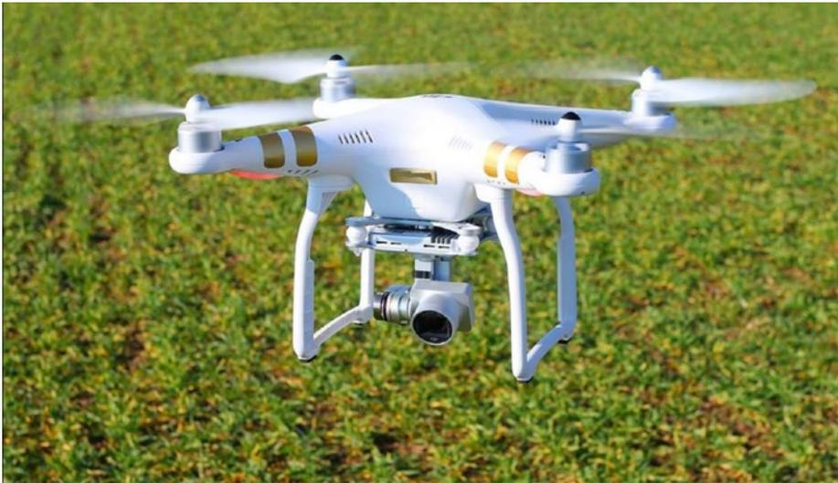
*Figure 2-4. An agriculture drone used to monitor crops*
