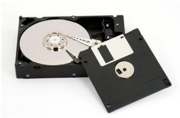
*Figure 3-2. Magnetic storage devices*
