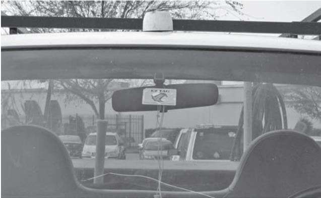
**FIGURE 25.5** Mounted passive E-ZPass tag.
