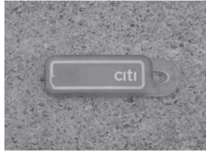
**FIGURE 15.2** RFID credit key fob.
