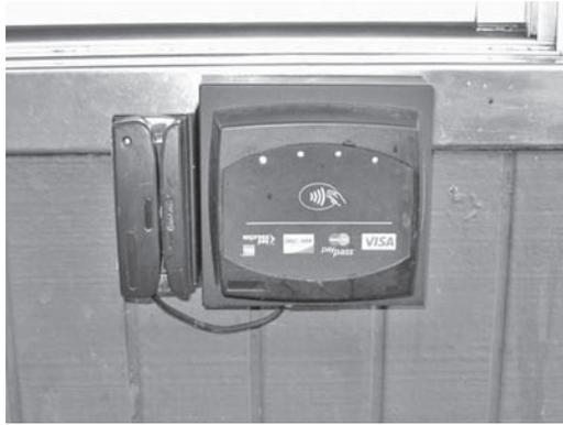
**FIGURE 2.3** Common type of RFID reader.
