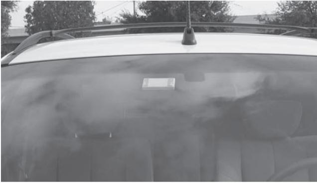
**FIGURE 25.3** EZ-Pass transponder mounted to car windshield.
