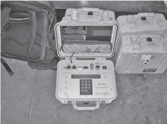
**FIGURE 23.5** Portable RFID reader.
