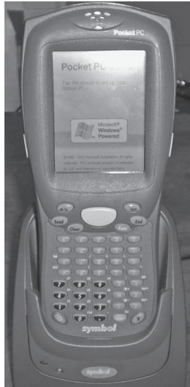
**FIGURE 2.10** Typical handheld RFID scanner.
