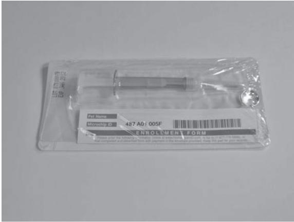
**FIGURE 14.4** Implantable RFID tag and injector.
