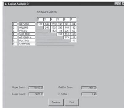
FIGURE 38.19 Screen display giving distances between departments for current layout.
