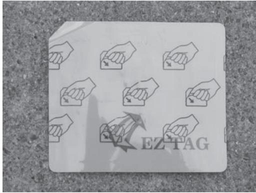
**FIGURE 25.4** Windshield-based RFID tag.
