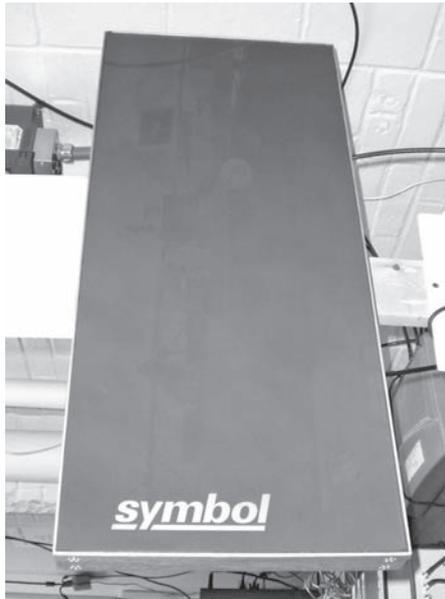
**FIGURE 3.23** AN400 high-performance area antenna.
