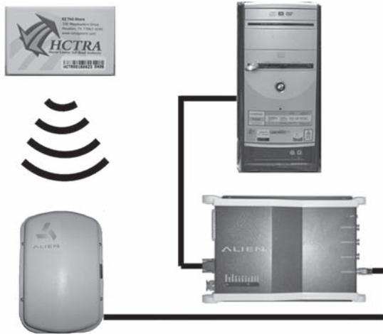
**FIGURE 2.1** Basic RFID system components.
